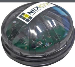
WixLi Zhaga™ is a low-profile, high performance node fitted for any luminaire equipped with Zhaga 18 socket. Compliant with DALI-1 and DALI-2 driver interface, WixLi Zhaga™ is available in ZigBee wireless interface.
